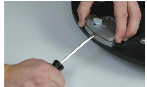
Strong earth magnets (3) secure the individual Trapezoid diamonds. A screwdriver is used to pry the trapezoid from the magnetic base.
